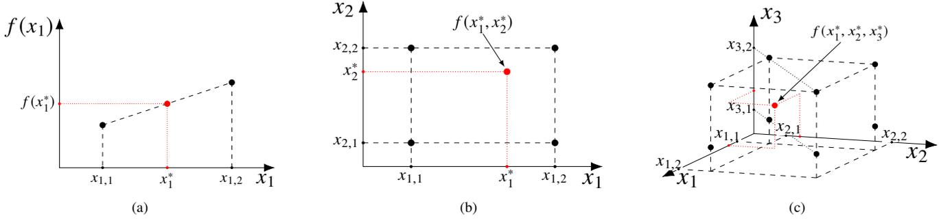
Fig. 1. Examples of regular grids for (a)  $D = 1$ , (b)  $D = 2$  and (c)  $D = 3$  showing the number of vertices surrounding the point where the interpolant must be calculated. The number of vertices surrounding a point  $x_i^*$ ,  $i = 1, \dots, D$  where the interpolant is to be calculated is  $2^D$ .
