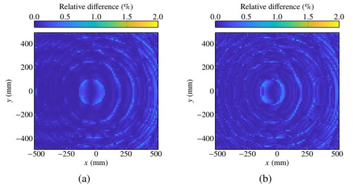
Fig. 3. For the reflectarray layout design, relative error of the layout for polarization X with regard to the design carried out with MoM-LP of the (a) LUT and (b) SVR.
