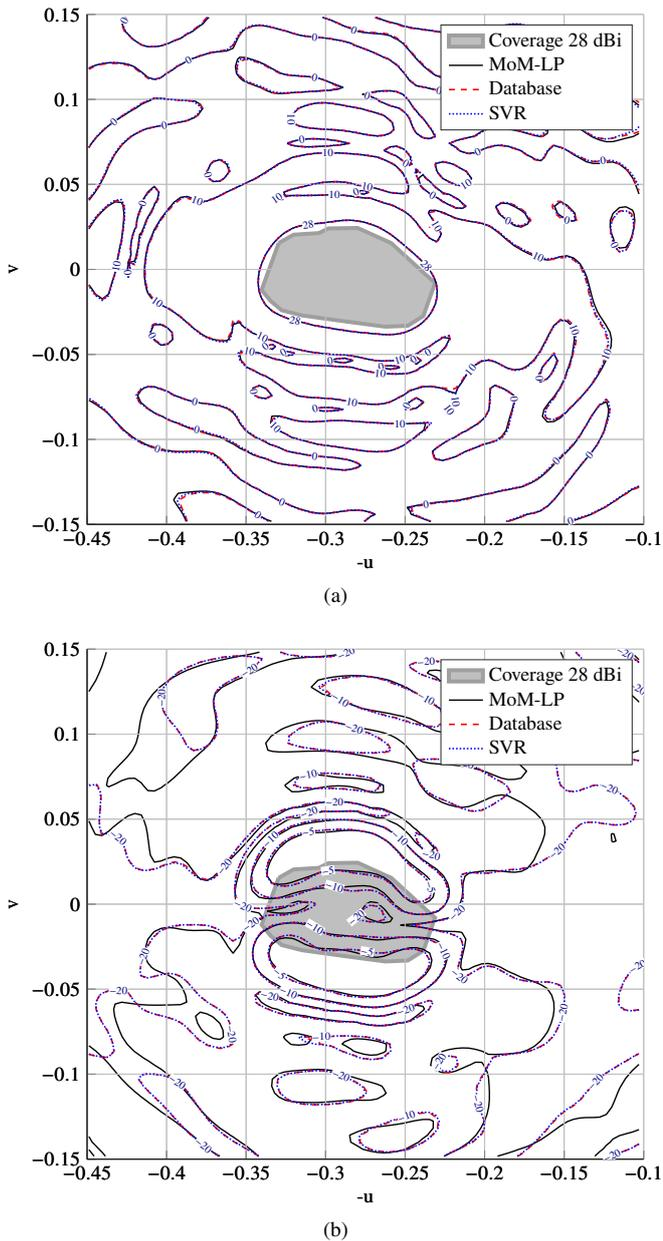
Fig. 4. Comparison of the simulations with MoM-LP, database and SVR for the (a) copolar and (b) crosspolar patterns for polarization X of a reflectarray with European coverage using a layout obtained with the database.
