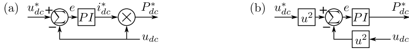
Figure 4.4: Implementation of the DC voltage control loop following (a) Direct Voltage Control (DVC) and (b) Quadratic Voltage Control (QVC) approaches.
