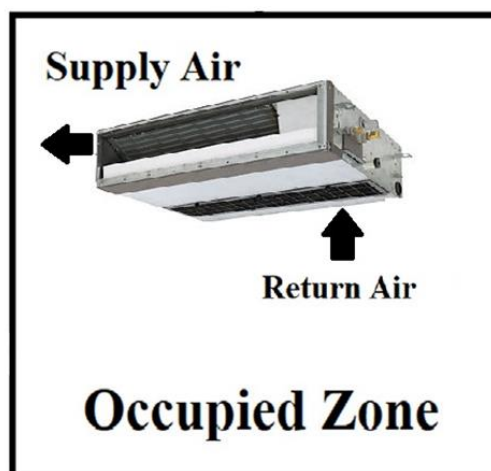
Figure 4-17: FCU system arrangement
