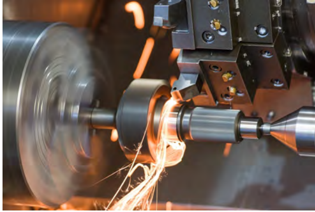
Figure 1.4.: Hard turning of a nickel-based alloy (Inconel 718) with the cutting material CBN [109]
