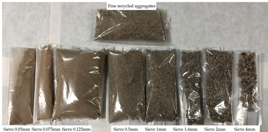
Fig. 2. Recycled Fine Aggregate with different sizes.
