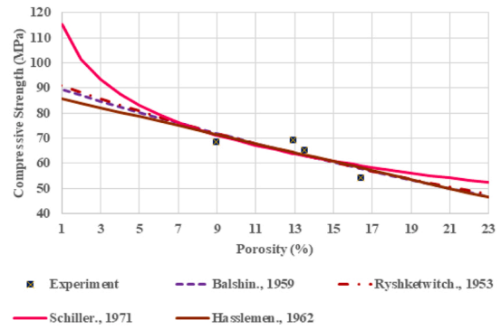
(b) Porosity Vs compressive strength at 90 days.
