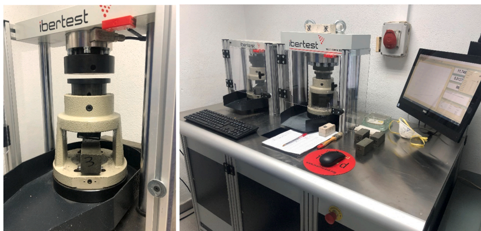
Fig. 3. Compressive and flexural strength test of RFA mortar.
