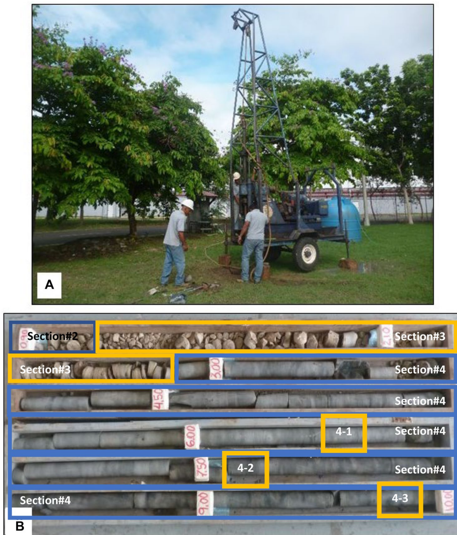
Fig. 4 Study area: (a) drilling of well; (b) lithological logs of drill cores. The different lithological sections described in the location of the three subsamples 4 are indicated
