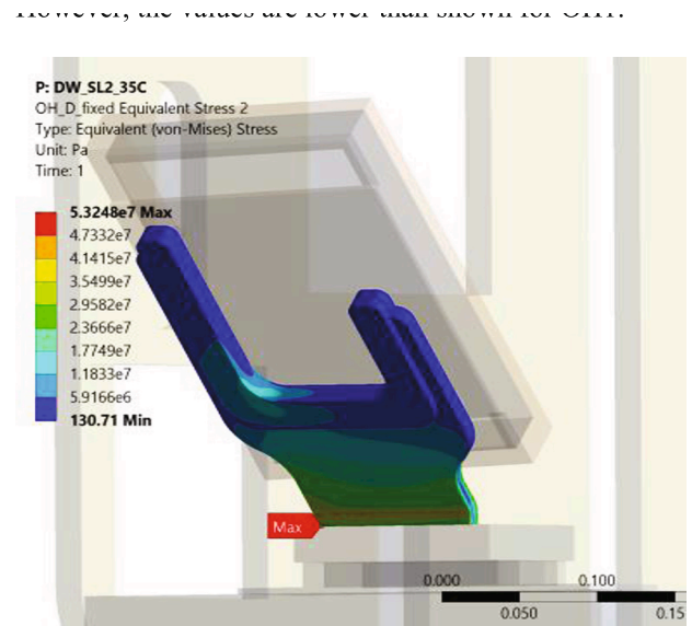
Fig. 16. OH2 maximum primary stresses in LCIV.1.
