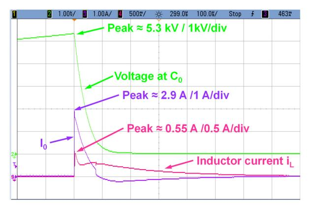
Figure 14. Waveforms at the output during breakdown.
