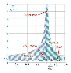
**Figure 4.** Voltage gain versus normalized switching frequency and the position of some operation points.
