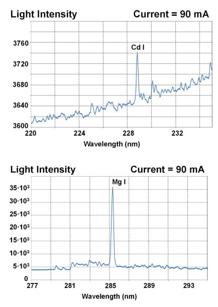
**Figure 15.** Experimental results of the system when measuring tap water containing a small quantity, 0.5 ppm, of Cd.
