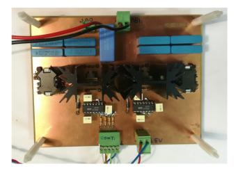
**Figure 5.** Inverter of a prototype. RM10 snubber inductors appear on the borders. PCB size has not been optimized.
