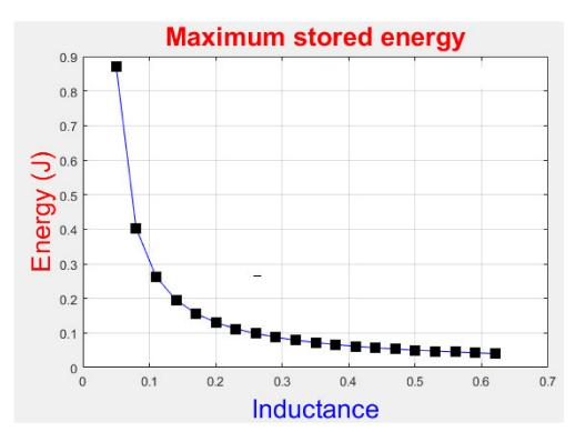
Figure 13. Stored energy at the inductor when the current through it reaches its maximum against inductance.
