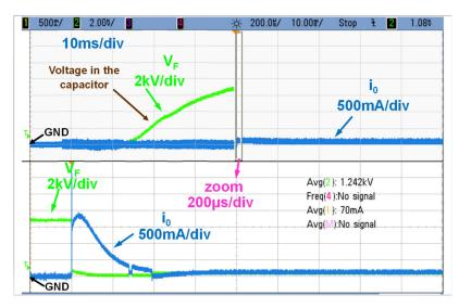
**Figure 9.** Output current,  $i_0$ , and capacitor voltage,  $V_F$ , evolution before and after breakdown when distance between electrodes is 3 mm.
