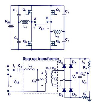
**Figure 2.** Parallel resonant converter with a capacitive output filter, PRC-C. An additional passive network,  $(L_1, L_2, C_1-C_4)$  is added to obtain soft switching in the whole inverter operating range.
