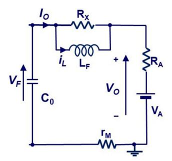
Figure 12. Second-order output filter to improve efficiency.
