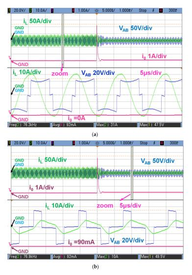
**Figure 10.** Inverter voltage,  $V_{AB}$ , resonant current,  $i_L$ , and output current,  $I_0$ , before (**a**), and after (**b**) breakdown.
