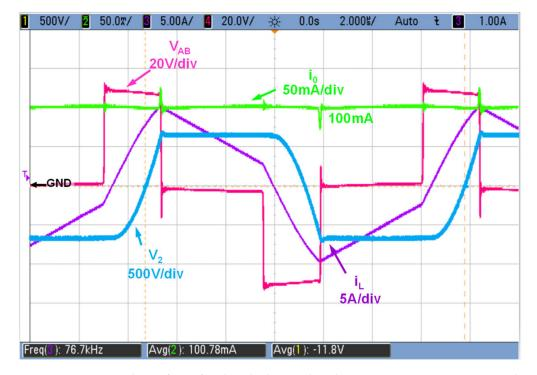
**Figure 7.** Experimental waveforms for glow discharge when the output current is 100 mA. Switching frequency is 76.7 kHz, d is 0.18 and V<sub>F</sub>, not in the image, is 632 V.
