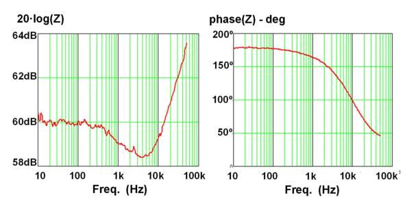
**Figure 6.** Experimental, small signal characterization of the glow-discharge impedance. This was obtained from dynamical measurements of the output voltage and current.
