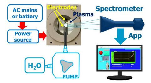
Figure 1. Conceptual scheme of the portable pollutant detector.
