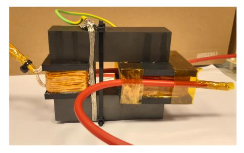
Figure 3. Step up transformer: left: primary winding; right: concentric high-voltage coils.
