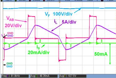
**Figure 8.** Experimental waveforms for glow discharge. Top:  $f_S = 76.5$  kHz, d = 0.39,  $i_0 = 170$  mA,  $V_0 = 693$  V. Bottom:  $f_S = 91.9$  kHz, d = 0.11,  $i_0 = 50$  mA,  $V_0 = 627$  V.
