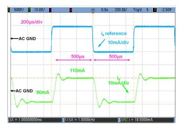
**Figure 11.** Dynamic response of the output current facing a change in the reference every 500 μs.
