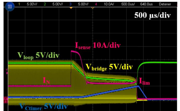
Fig. 16. Class 10 LCL operation under a short-circuit for a V bus of 100V, using the ROHM N-MOSFET
