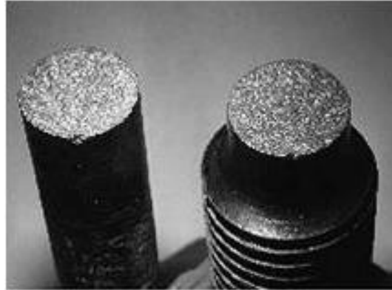
FIGURE 1.9.- Examples of brittle fractures
