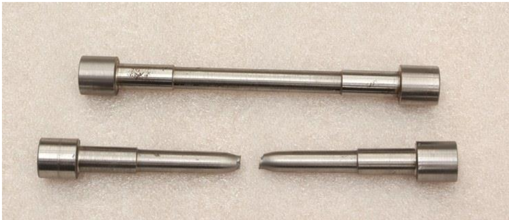
FIGURE 2.3.- Ductile fracture after axial load test
