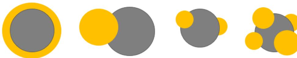
**Figure 2.** Schematic illustration of the different dual nanoparticle architectures where the grey ball represents the SPIONs and the yellow one represents the noble metal nanoparticle. From left to right: core-shell and a dumbbell-like nanoparticle while the other two represent the structure of a nanoflower with two and four domains.
