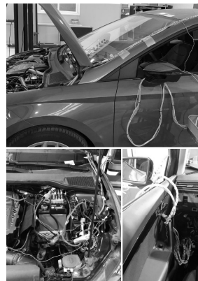
Fig. 10. Vehicle fuse boxes with measuring probes.
