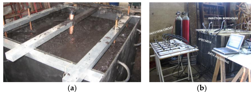
Figure 2. (a) Preparation of the coal sample for CO 2 generation tests. (b) Set-up of the equipment for the CO 2 generation tests at a medium scale.
