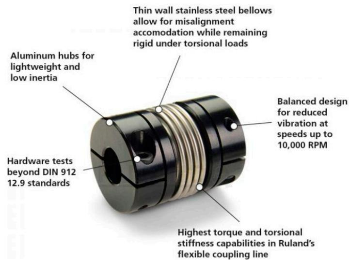
**Figure 26.** Flexible coupling properties (main features).
