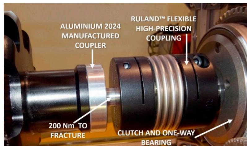
**Figure 27.** Flexible coupling properties (detailed view).
