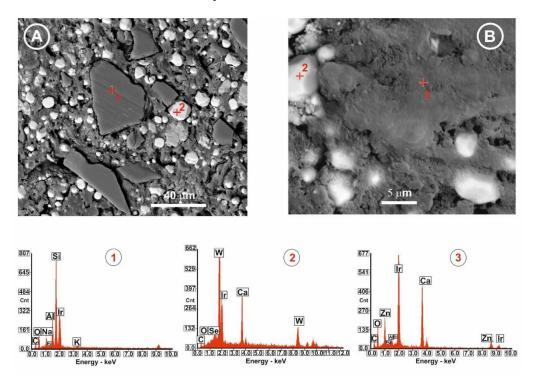
**Figure 6.** (**A**,**B**) Backscattered FE-SEM micrographs; (**1**,**2**,**3**) EDS microanalysis, of the selected spots (red cross with the corresponding numbers) of the dental sealer containing the bactericidal materials, (**A**) G3T glass-ceramic and (**B**) ZnO-enriched glass, both located at the delta apical of the canal.
