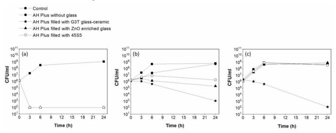
**Figure 1.** Antibacterial activity of glass-filled AH Plus: (a) Samples were used within 20 min after mixing; (b) samples were allowed to set for 48 h in a humid atmosphere at 37 °C; (c) samples were allowed to set for 48 h in a humid atmosphere at 37 °C, and then aged for 5 days in phosphate buffered saline (PBS) at 37 °C. All the assays were conducted in triplicate, each point on the curve is the average of three measures.
