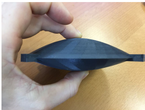
Figure 3.37: Final prototype of the doubly hyperbolic lens after removing the PVA support.
