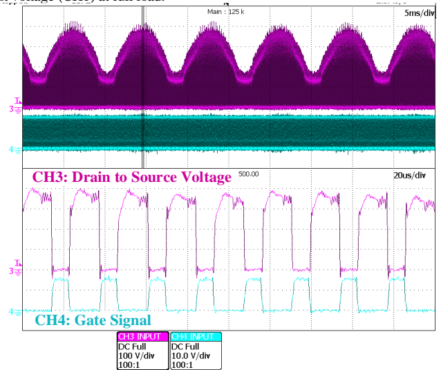
Fig. 14. Gate-to-source signal (CH4) and drain-to-source voltage across of the MOSFET (CH3).
