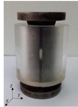
Figure 4. Tensile device plus sample.
