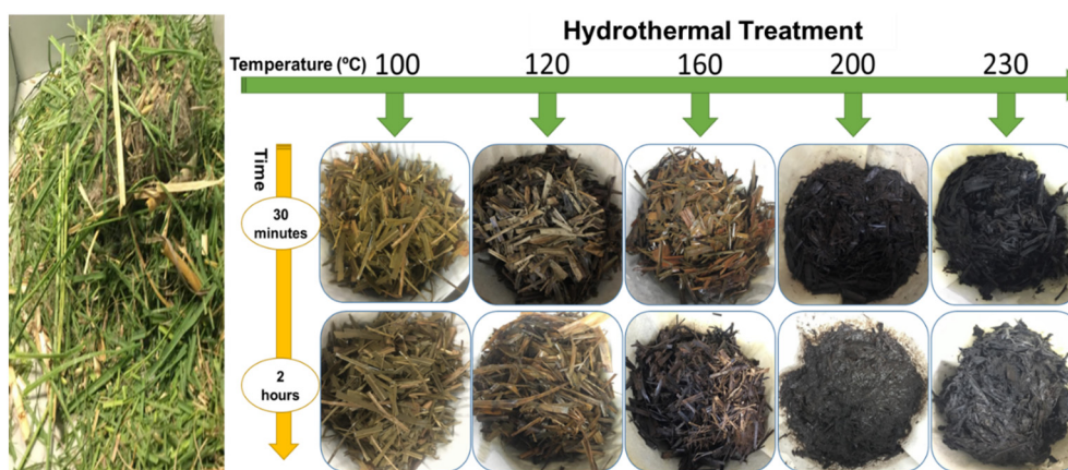
Fig. 1. Pampas grass waste and the solid products obtained by hydrothermal treatment under different conditions.
