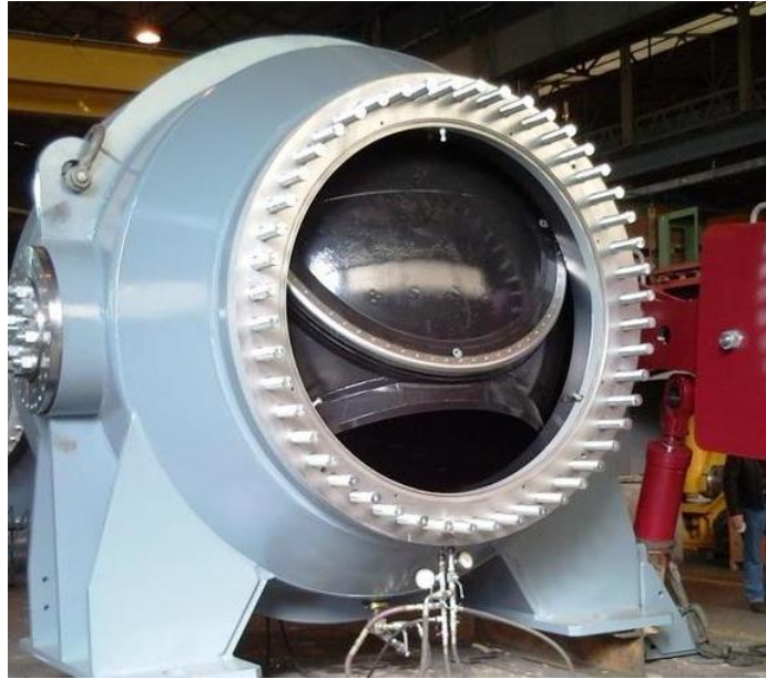
Figure 1.4: A partially opened spherical valve ( Vortex Hydra Dams, 2021 ).
