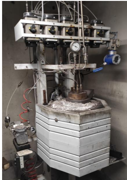
Figure 3.7. High-pressure hydrogen reactor used to pre-charge the steel samples. It is located in Idonial Technology Centre, Asturias, Spain.
