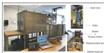
Fig. 5. Descriptive photographs of the hydrodynamic tunnel.
