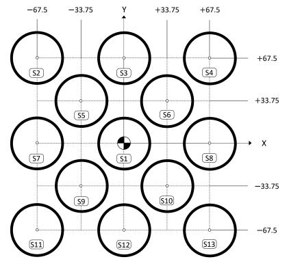
Figure 3. Distribution of parts according to the selected thirteen states in the manufacturing tray.
