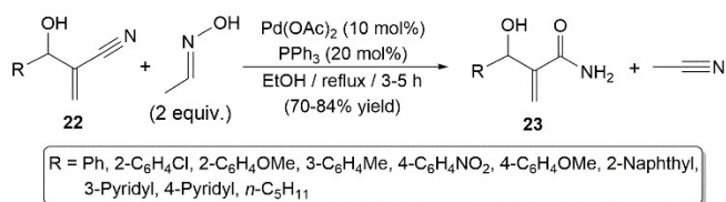
Scheme 22. Pd-catalyzed transfer hydration of \beta -hydroxynitriles 22 .
