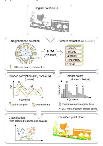
**Figure 6.** Workflow of the proposed methodology to select the optimum scales (impact points) and perform the multiscale classification.
