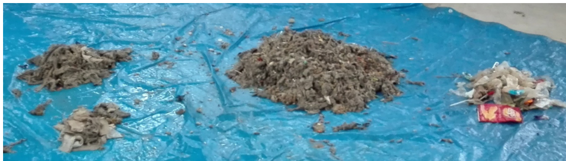
Figure 3. Gross solids sample removed in pretreatment at Villapérez WWTP.
