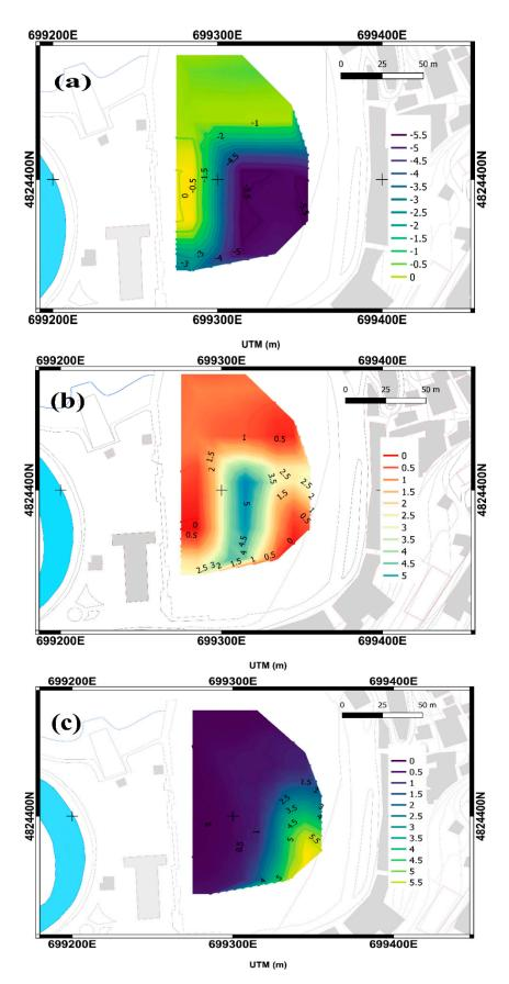
**Figure 7.** Difference in elevation of the bathymetries in the Port of Luarca between (**a**) 16/11/18 and 31/12/18, (**b**) 31/12/18 and 05/01/19, and (**c**) 05/01/19 and 24/02/19.
