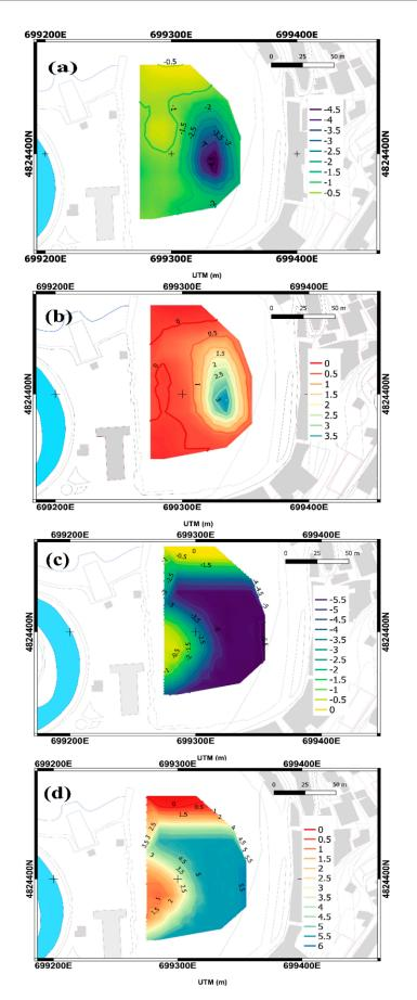
**Figure 6.** Difference in elevation of the bathymetries in the Port of Luarca between (**a**) 02/09/17 and 20/10/17, (**b**) 02/10/17 and 02/11/17, (**c**) 21/11/17 and 21/12/17, and (**d**) 21/12/17 and 24/02/18.
