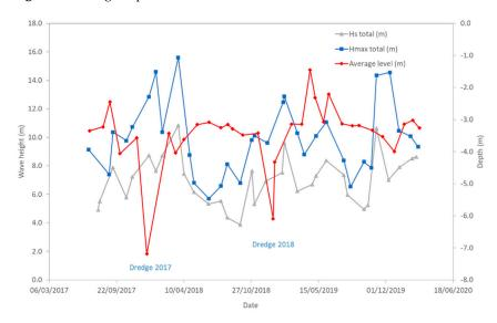
Figure 9. The effect of the wave height (H) on the average level of the dock in the Port of Luarca.
