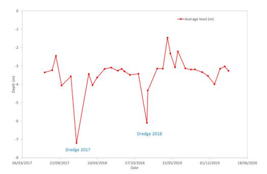
Figure 8. Average depth of the bottom of the dock in the Port of Luarca.
