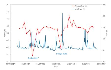
Figure 10. Effect of the Negro River on the average level of the dock in the Port of Luarca.
