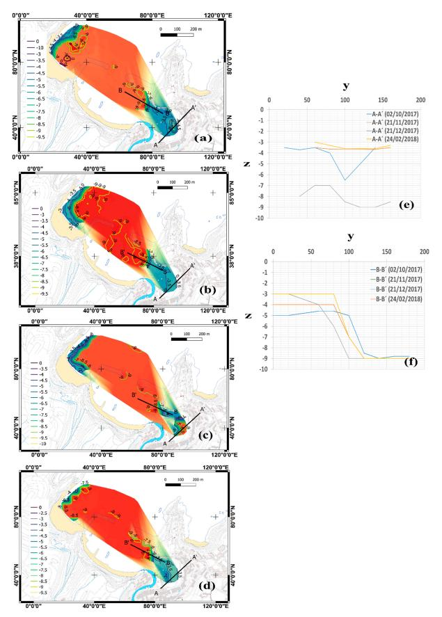
**Figure 5.** A representation of the behavior of the interior basin the dredging on: (a) 02/10/17, (b) 21/11/17, (c) 21/12/17 and (d) 24/02/18; and cross-sectional profile (e) AA' of the inner dock, and (f) BB' of the inlet channel.
