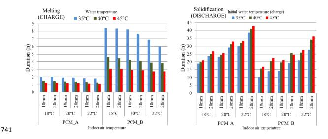
Figure 9. Melting and solidification times for PCM floors according the temperature of
