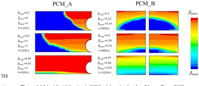
Figure 4. Melted liquid fraction in PCM subdomains for  $th_c = 20$  mm,  $T_{iair} = 20^{\circ}$ C,
