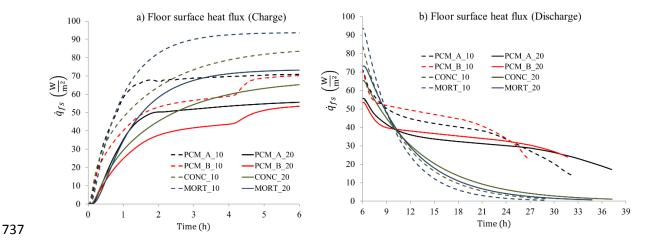
**Figure 8.** Evolution of the averaged heat fluxes at the surfaces of the radiant floors for  $T_{iair} = 20^{\circ}$ C and  $T_{hp} = 40^{\circ}$ C as a function of the cover thickness: a) charging b) discharging.
