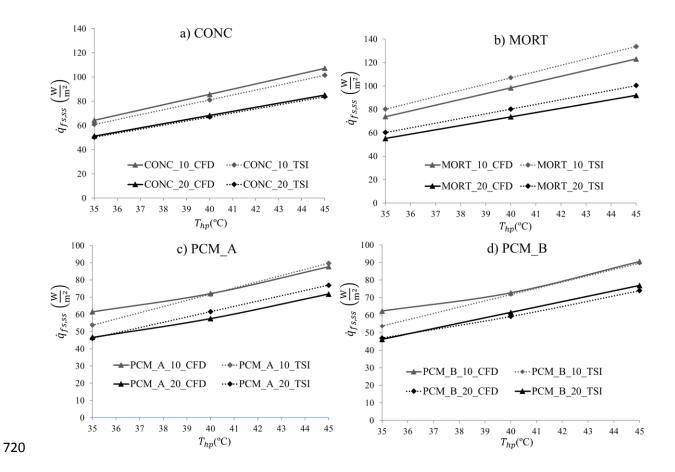
**Figure 3.** Steady-state heat transfer rates computed by CFD and TSI (proposed by ASRHAE) procedures for  $T_{iair}$ =20°C.
