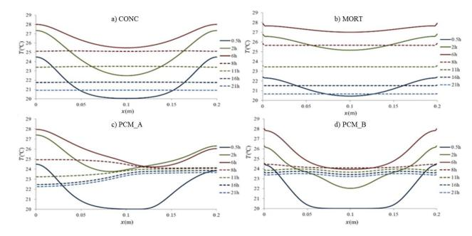
Figure 6. Temperature distribution during the discharge at points on the surface of the radiant floors for  $th_c = 20$  mm,  $T_{iair} = 20^{\circ}$ C,  $T_{hp} = 40^{\circ}$ C.
