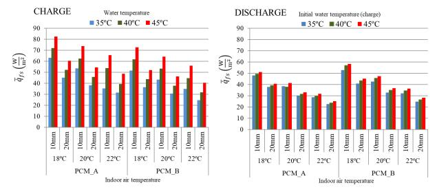
Figure 10. Time-averaged heat fluxes at floor surface during charging and discharging
