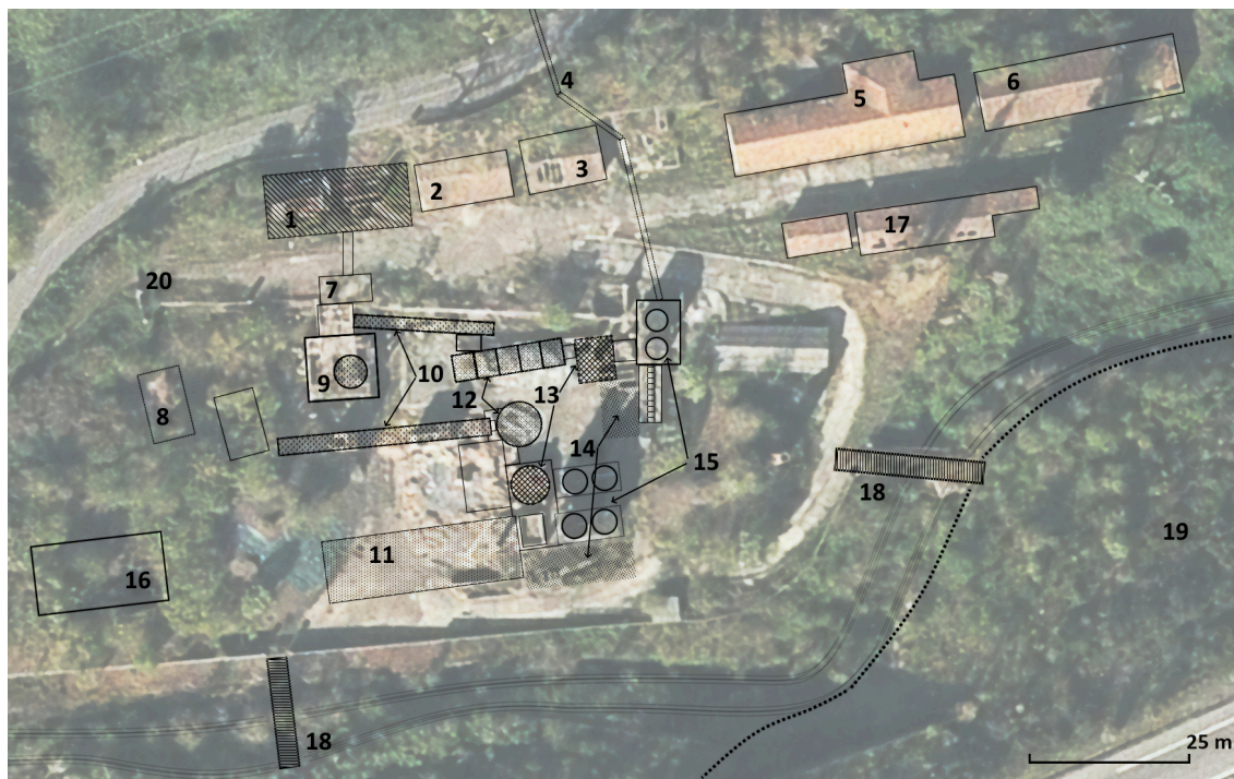
Figure 11.: Schematic view of the former location of known industrial installations and auxiliary buildings, overlaid with a recent satellite image. (1) Esperanza mine headframe. (2) Draw-works machinery. (3) Electric facilities. (4) Flue duct. (5) Offices and laboratories. (6) Dining room and lockers room. (7) Ore grinding and sorting station. (8) Furnace fuel storage tanks. (9) Herreshoff kiln. (10) Rotary furnaces. (11) Muffle-type furnace. (12) Arsenic condensers. (13) Mercury condensers. (14) Waste treatment areas. (15) Mercury and mercury soot condensation tanks. (16) Workshop and carpentry area. (17) Storage buildings. (18) Bridges across San Tirso river. (19) Large spoil heap, currently buried under the AS-I motorway. Satellite imagery obtained via ArcGIS web server using World Imagery map layer and upscaled using ISR (Cardinale et al., 2018). Map sources: Esri Community Maps Contributors, Dirección General de Catastro, CC-BY 4.0 scne.es, Esri, HERE, Garmin, INCREMENT P, METI/NASA, USGS.
