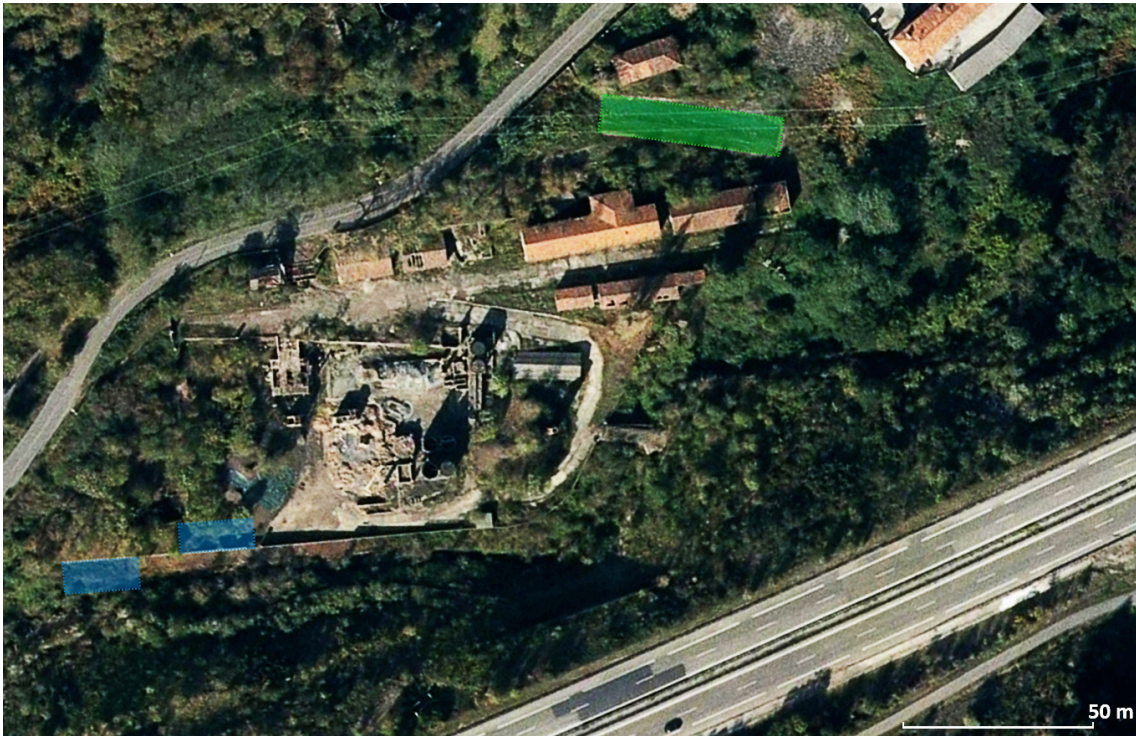
Figure 14.: Location of remediation plots within the site overlaid with a satellite image. Green: phytoremediation; blue: soil stabilisation with zero valent iron nanoparticles. Satellite imagery obtained via ArcGIS web server using World Imagery map layer and upscaled using ISR (Cardinale et al., 2018). Map sources: Esri Community Maps Contributors, Dirección General de Catastro, CC-BY 4.0 scne.es, Esri, HERE, Garmin, INCREMENT P, METI/NASA, USGS.
