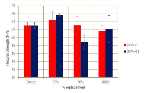
Figure 9. Flexural strength of UHPFRC for both wastes (GCW-D [14] and GCW-GS).
