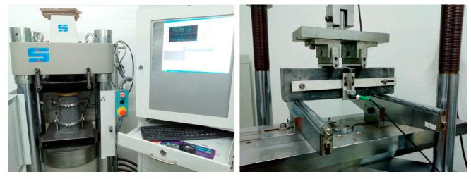
Figure 4. Modulus of elasticity and flexural strength tests.
