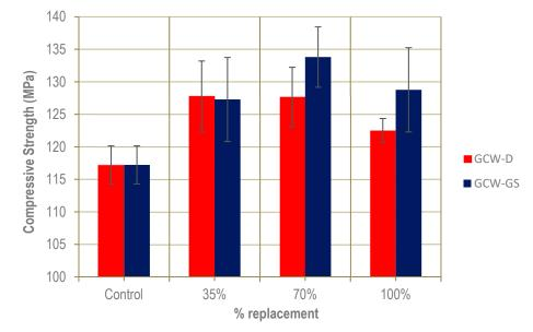
Figure 7. Compressive strength of UHPFRC for both wastes (GCW-D [14] and GCW-GS).
