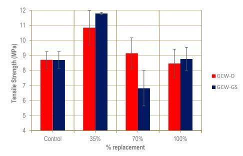
Figure 11. Tensile strength of UHPFRC for both wastes (GCW-D [14] and GCW-GS).
