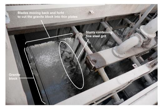
Figure 1. Granite gang saw cutting machine.
