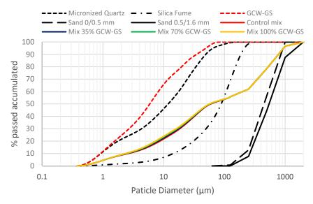
Figure 2. Granulometric curves of materials and resulting mixes.
