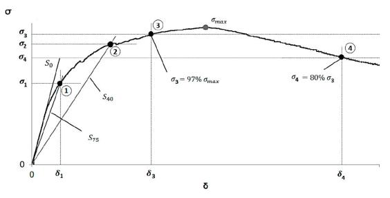
Figure 10. Stress-strain curves and key points.
