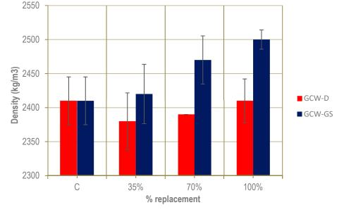
observed, the variation is less than 2% and is within the error bars (Figure 6). In summary, the incorporation of GCW-GS produced an increase in the density of the concrete while the incorporation of the residue GCW-D did not affect this property.
