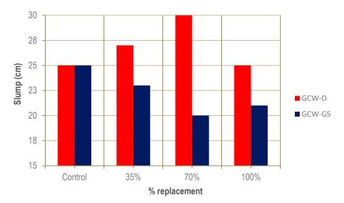
Figure 5. Slump of UHPFRC for both wastes (GCW-D [14] and GCW-GS).
