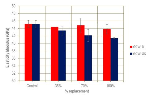
Figure 8. Elasticity modulus of UHPFRC for both wastes (GCW-D [14] and GCW-GS).
