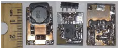
Fig. 10. Transmitter prototype: passive board (top view), GaN-FET board (top view) and passive board (bottom view).
