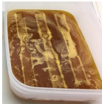
Figure 2. Formation of hydrogen bubbles after immersion in ferric chloride solution
