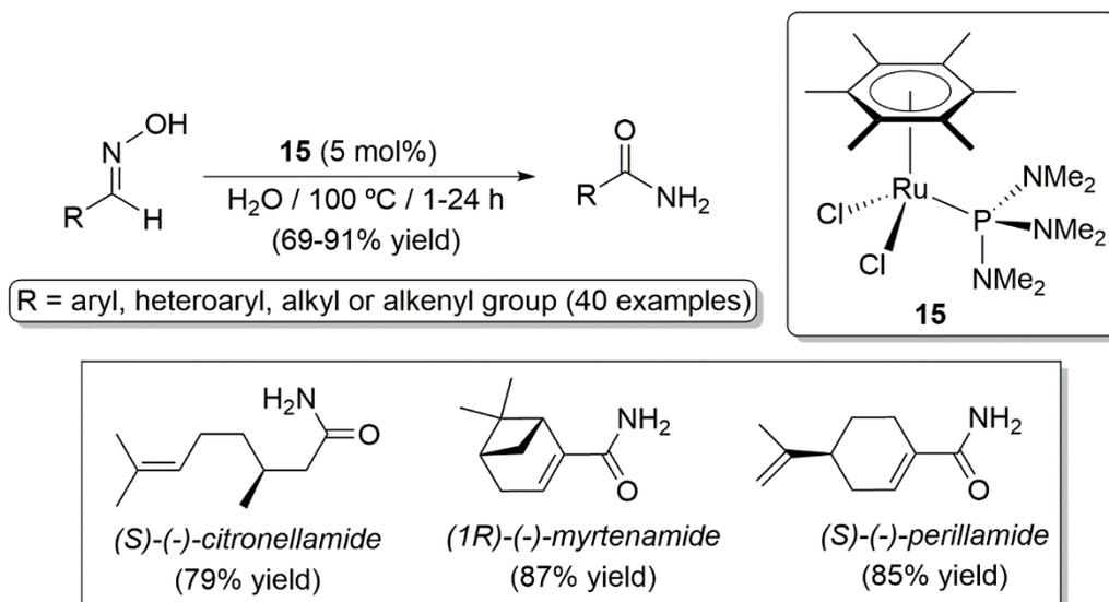
**Scheme 23.** Catalytic rearrangement of aldoximes in water using complex **15** as catalyst.
