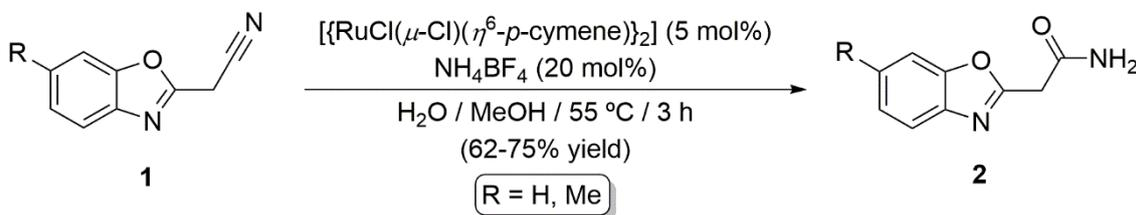
**Scheme 3.** Hydration of benzoxazolylacetonitriles **1** employing dimer  $[\{\text{RuCl}(\mu\text{-Cl})(\eta^6\text{-}p\text{-cymene})\}_2]$ .
