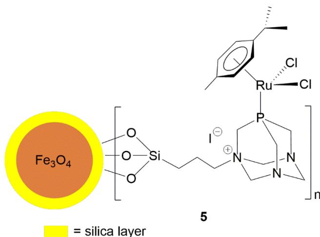
**Fig. 2.** Structure of the ruthenium nanocatalyst **5**.
