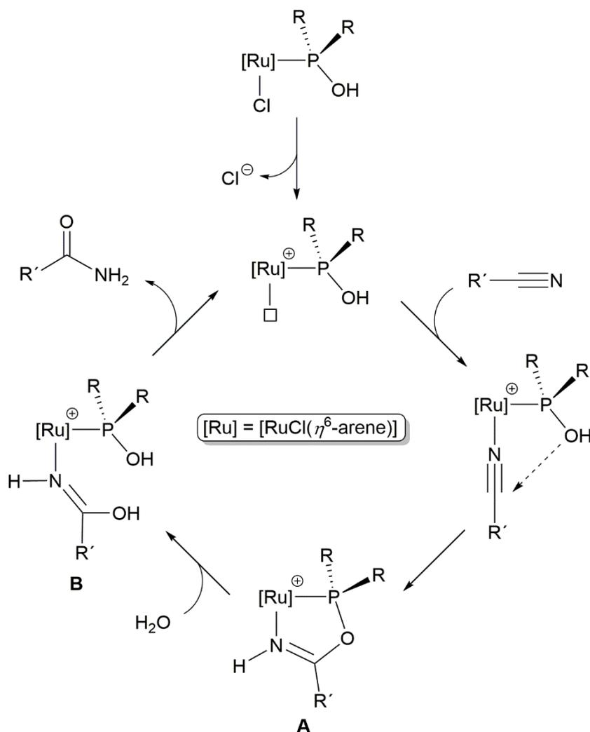
**Scheme 12.** Mechanism for the hydration of nitriles catalyzed by complexes  $[\text{RuCl}_2(\eta^6\text{-arene})(\text{PR}_2\text{OH})]$ .
