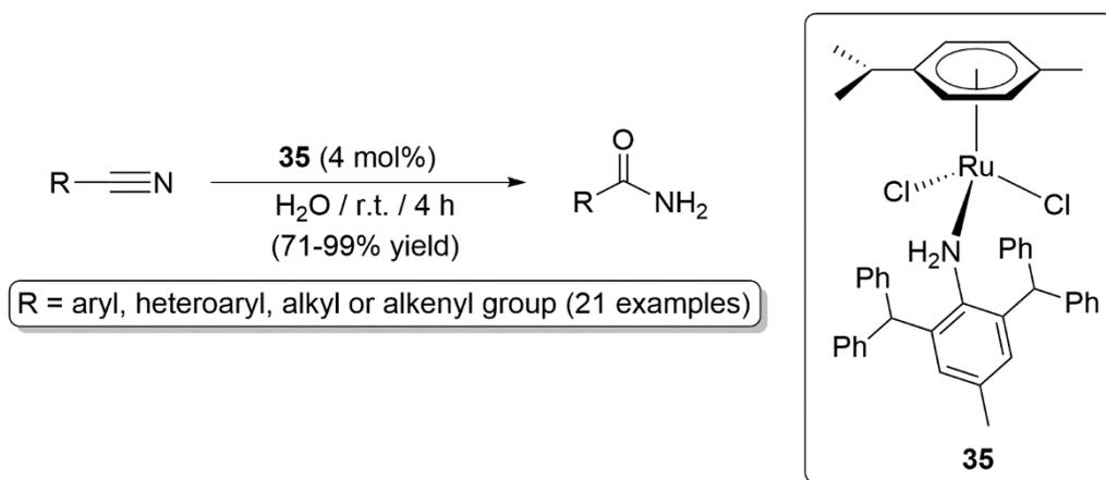
**Scheme 18.** Nitrile hydration reactions catalysed by the superbulky water-soluble complex **35**.
