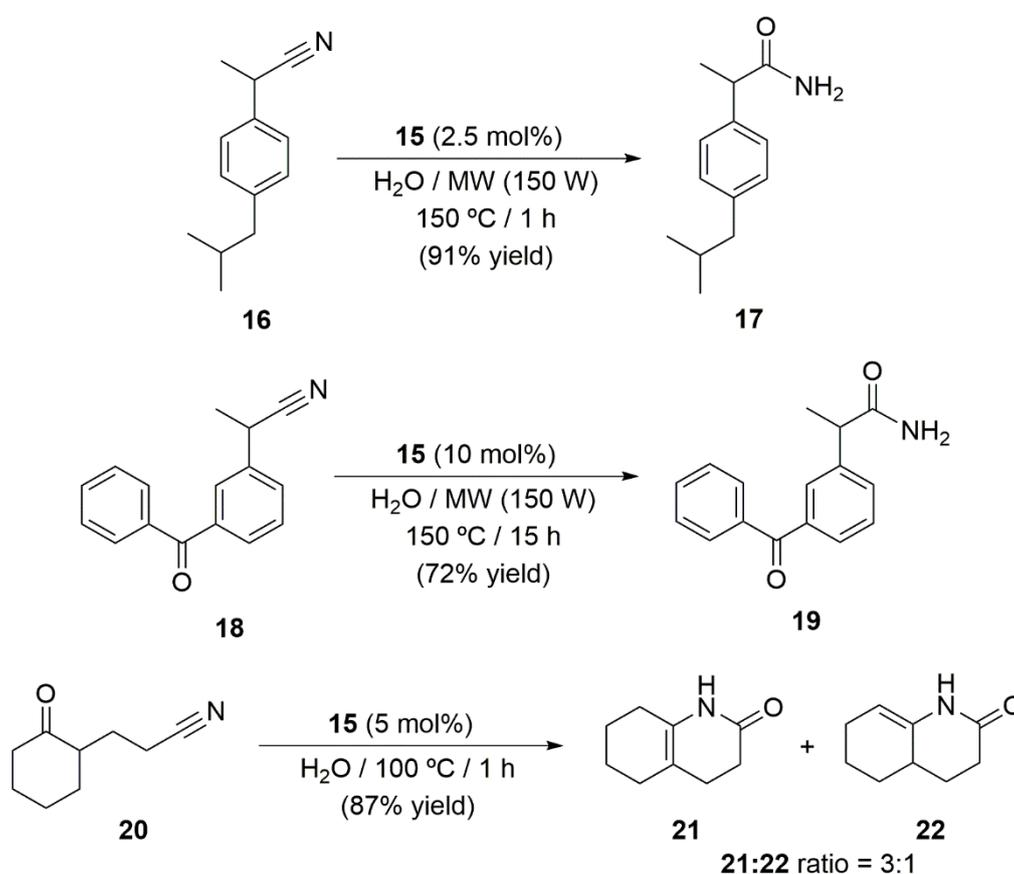
**Scheme 10.** Access to ibuprofenamide, ketoprofenamide and ene-lactams using  $[\text{RuCl}_2(\eta^6\text{-hmb})\{\text{P}(\text{NMe}_2)_3\}]$  (**15**) as catalyst.
