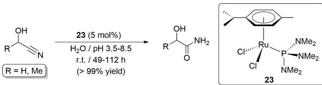
**Scheme 11.** Catalytic hydration of glycolonitrile and lactonitrile using complex [RuCl<sub>2</sub>( $\eta^6$ -*p*-cymene){P(NMe<sub>2</sub>)<sub>3</sub>}] (**23**).
