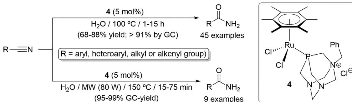
**Scheme 5.** Nitrile hydration reactions with the water-soluble complex [RuCl<sub>2</sub>( $\eta^6$ -hmb)(PTA-Bn)] (**4**).
