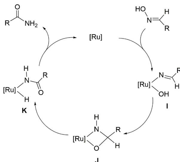
**Scheme 26.** Catalytic synthesis of primary amides from aldehydes catalysed by the dinuclear complex **47**.
