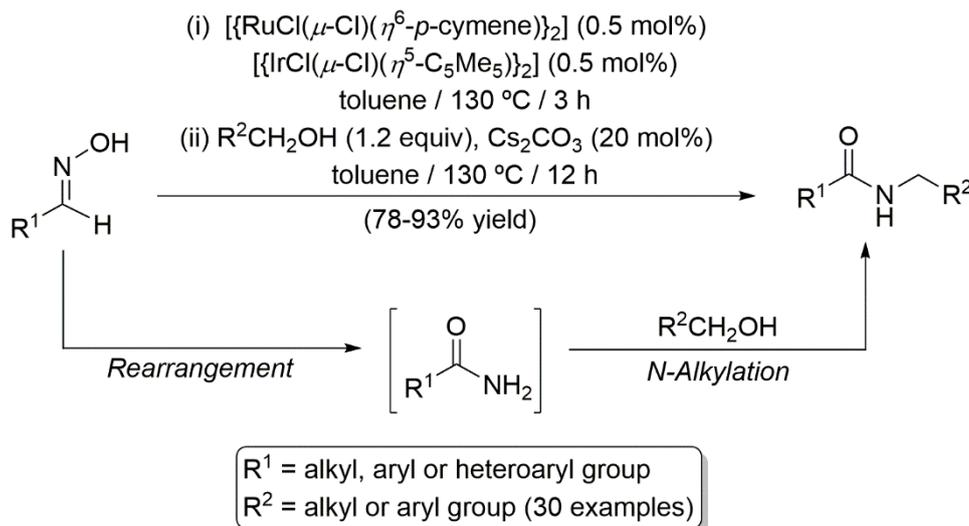
**Scheme 28.** Catalytic synthesis of secondary amides from aldoximes and primary alcohols.
