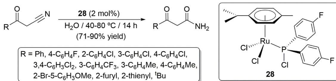
**Scheme 14.** Catalytic hydration of  $\beta$ -ketonitriles using the arene-Ru(II) complex **28**.
