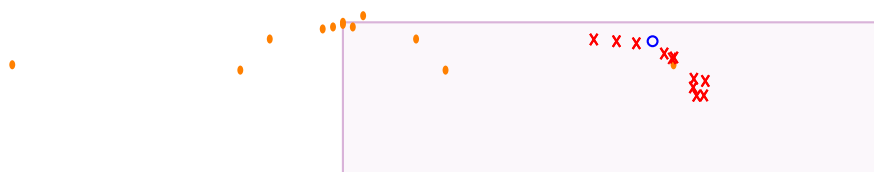
Fig. 2 Graphical representation of the dimer problem. The orange points are the 12 poles of the rational function. The shaded part is the region used in the NLEIGS solver, while the blue circle is the target value used in both NLEIGS and SLP. Red crosses are the 20 eigenvalues computed by NLEIGS (there are more eigenvalues inside the region).
