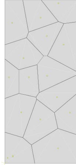
Figure 6. Synthetic microstructure generated by Voronoi tessellations to reproduce the sample T_g = 1100^\circ\text{C} , and the corresponding histogram of grain size distribution.
