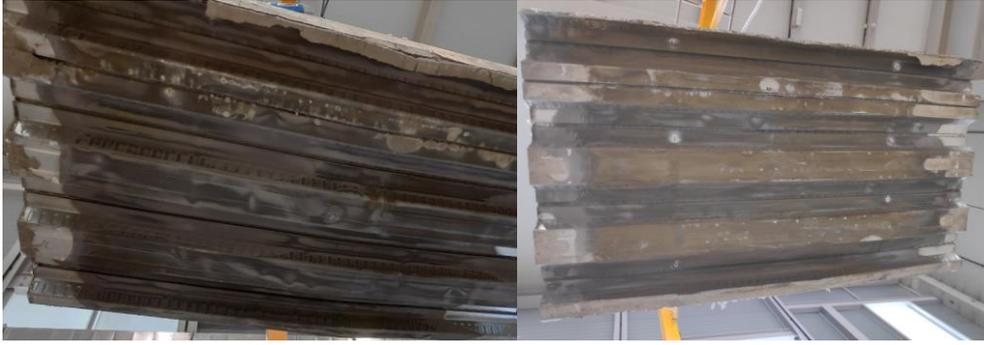
Fig 32. Disappearance of the zinc and the oxidation of the steel decking at the end of the test.
