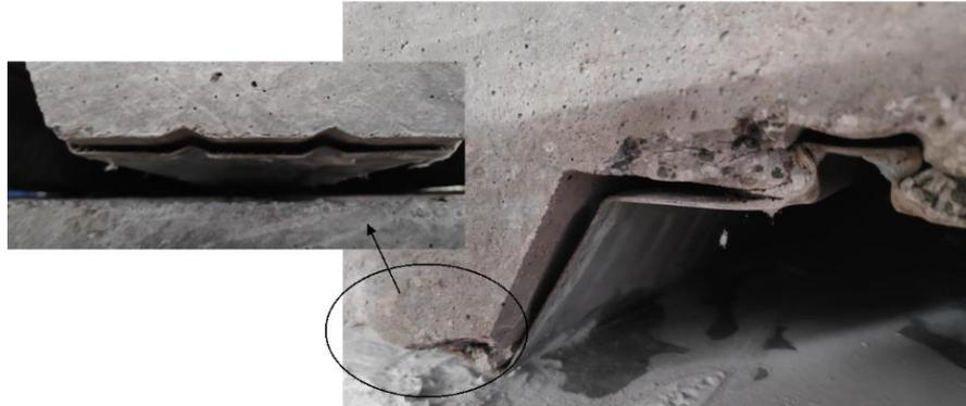
Fig 36. Debonding between steel and concrete.
