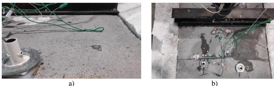
Fig 31. Water expelled during the test on the unexposed side of the slab: a) At the beginning of the test; b) At the end of the test.
