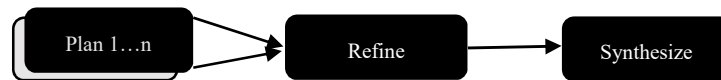
Fig. 1. The phases of a meta-planner to realize a multi-robot path with no collision.
