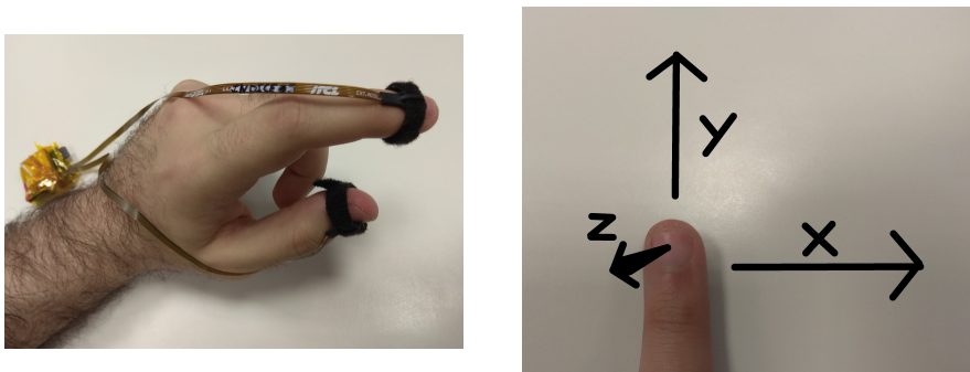
Fig. 1: Left part: The prototype sensing unit, with two 3DACC located on each finger end. Right part: 3DACC axes orientation relative to its finger. The z -axis is perpendicular to the finger, positive to the outside of the hand.
