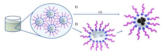
**Figure 8.** Schematic view of the synthesis of the magnetic nanoparticles studied. Water-based solutions of the iron precursors are used to form a microemulsion in the oil phase. The precipitation of the particles is achieved by means of the dropwise addition of either (1) the basic ammonia solution or (2) another microemulsion containing the ammonia.
