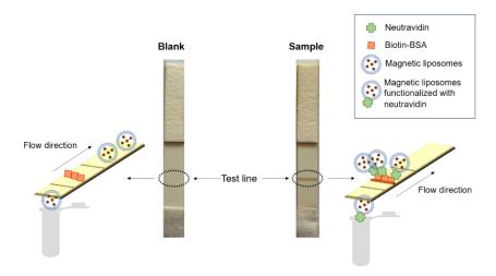
Figure 5. Scheme of affinity lateral flow assay using magnetic liposomes as labels.
