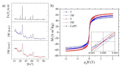
**Figure 4.** (a) XRD spectra obtained from the samples 3W and 5W compared with the magnetite pattern Puritronic<sup>®</sup>. (b) Magnetization curves at room temperature for the samples 3 and 5 before (3, 5) and after the washing procedure (3W, 5W). Inset: central area detail of the magnetization curves for the samples obtained by co-precipitation, CoP5, and ME.
