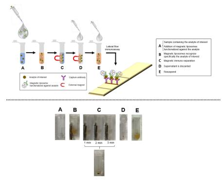
**Figure 6.** Process of immuno-separation, including the different steps schematically and with photographs. (**A**) Solution with the analyte. (**B**) Immuno -separation with a conventional magnet using magnetic liposomes. (**C**) Immuno-separation after 1 min, 2 min and 3 min. (**D**) Pellet after immune-separation. (**E**) Pellet resuspended with buffer.
