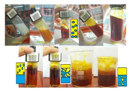
**Figure 7.** Evolution of the microemulsion system CTAB-1butanol-1hexanol with the increasing water phase content. A schematic view of the vial is showed for better understanding of the phases formed while the aqueous phase was added during titration.
