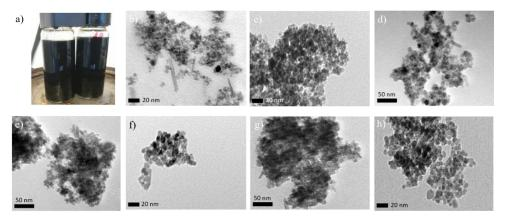
Figure 3. (a) Picture of the SPIONs synthesized and TEM images of the samples (b) 3, (c) 3W, (d) 5B, (e) 5, (f) 5W, (g) 5M and (h) CoP5.
