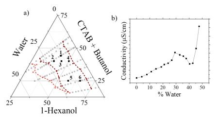
**Figure 1.** (a) Ternary diagram of the CTAB-butanol–hexanol–water system showing the composition of the different microemulsions used for the synthesis of the SPIONs, denoted as 1, 2, 3, 4, 5 and 6, all of them within the microemulsion stability region. (b) Conductivity measurements as a function of the water content for the point 6 in the CTAB-butanol-hexanol microemulsion system.
