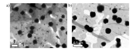
**Figure 2.** TEM images of the W/O microemulsions negatively stained with 1% phosphotungstic acid. Microemulsion with a composition corresponding to the formulations (**a**) 3 and (**b**) 5 in the ternary diagram of the CTAB-butanol–hexanol-water system.
