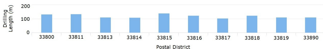
Figure 9. 100 m 2 building in Cangas del Narcea. Drilling length required for each postal district.
