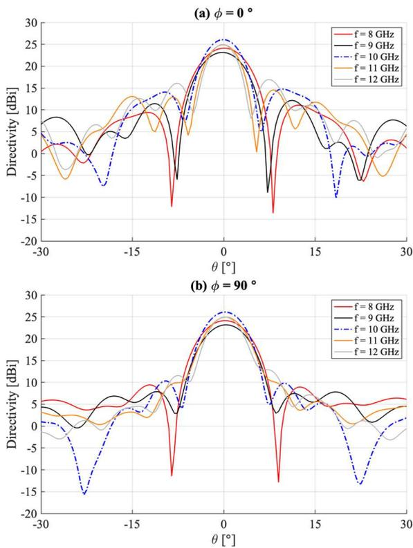
Fig. 6. Variation of measured directivity (co-polar component) through the X-band in the main planes. a)  $\phi = 0^\circ$  (H-Plane) and (b)  $\phi = 90^\circ$  (E-Plane).
