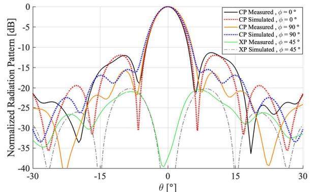
Fig. 5. Representation of the main planes of the measured and simulated radiation patterns, where  $\phi = 0^\circ$  (H-Plane) and  $\phi = 90^\circ$  (E-Plane).
