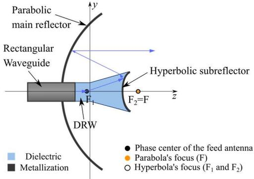
Fig. 1. Cassegrain antenna using the proposed self-supported subreflector, showing its side view. Also, it is represented the path through the structure of one example ray (in blue).
