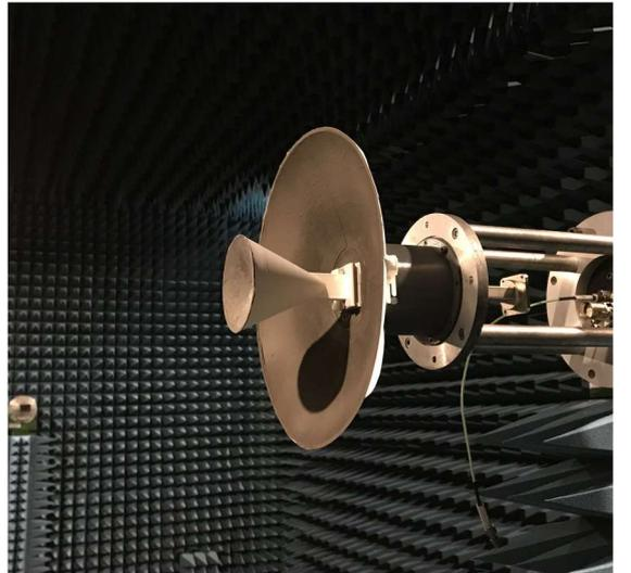
Fig. 3. Manufactured dual-reflector antenna using the novel subreflector in the measurement setup.
