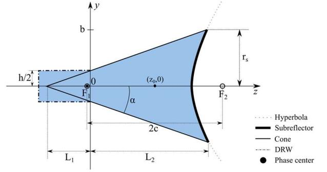
Fig. 2. Side view of the self-supported subreflector and feeding system, showing its geometric characterization.
