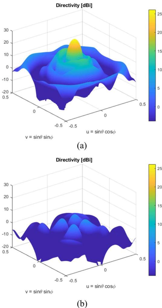
Fig. 4. 3-D representation of the measured radiation pattern at 10 GHz at (a) Co-polar component and (b) Cross-polar component.
