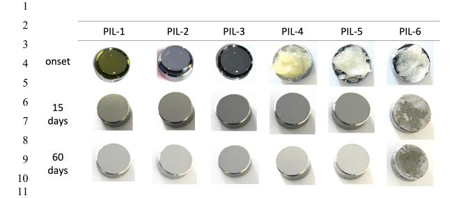
Finally, the surface topography of the disks exposed to the PILs was analyzed using a confocal microscope (Leica 3D) and the surface roughness was measured. Fig. 5 shows the corrosive effect of the PIL-6 on the disk surface topography.
