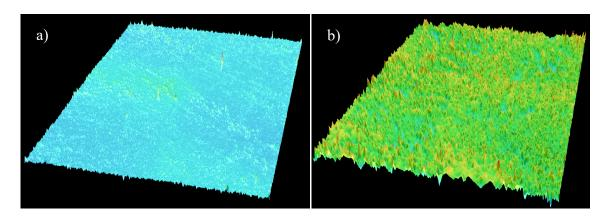
Fig. 5. Surface topography of fresh disk (a) and disk exposed to PIL-6 after 60 days (b).
