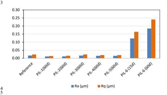
Fig. 6. Surface roughness of steel disks exposed to PILs (ISO 4287).
