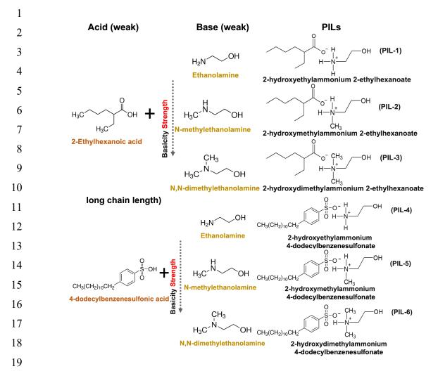
Fig. 1. Simplified procedure of synthesis of each PIL.
