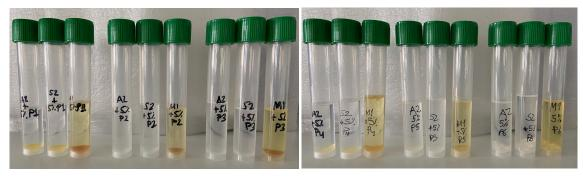
Fig. 7. Visual miscibility test (mixtures at 5.0 wt.% of PIL).
