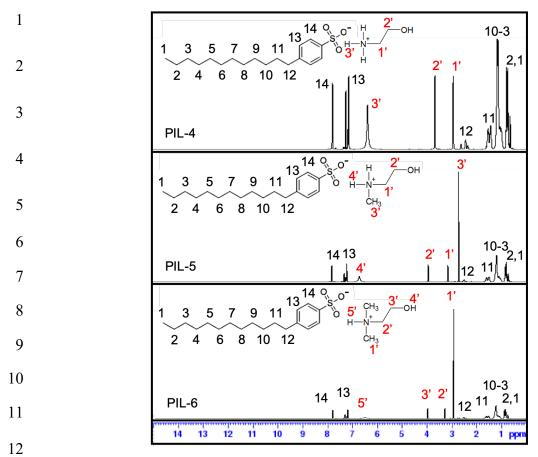
Fig. 2. <sup>1</sup>H NMR spectra of sulfonate-based PIL-4, PIL-5, and PIL-6.
