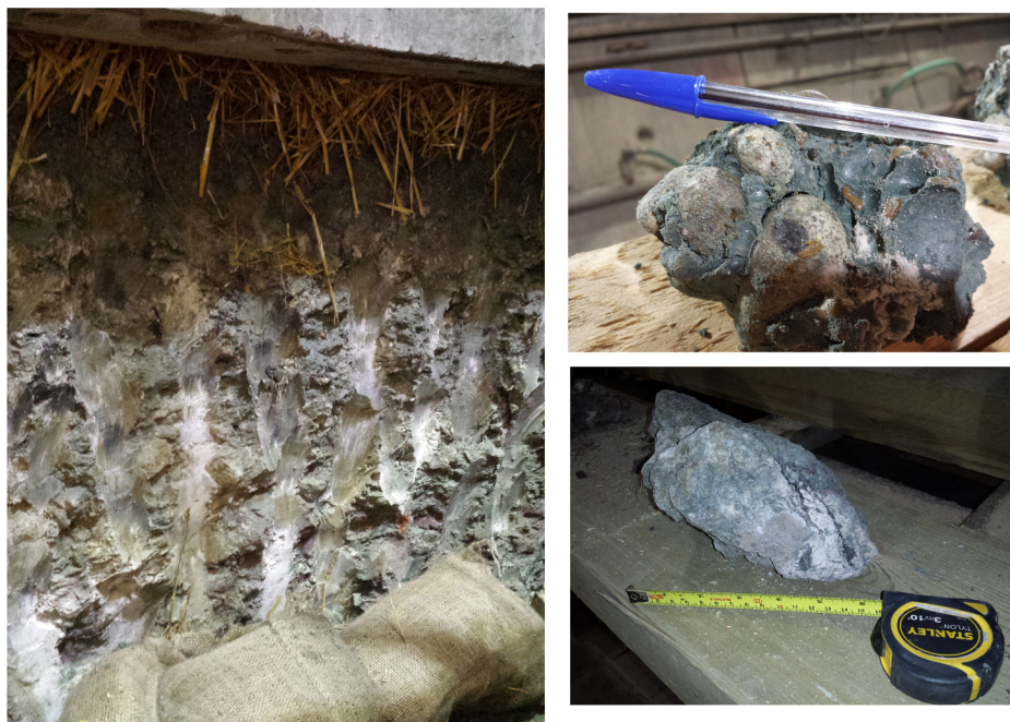
Fig. 22. View of some calcrete from the Lower Mottled Beds (left and right below) and the Upnor Formation conglomerate exposed in the cross passage sump.
