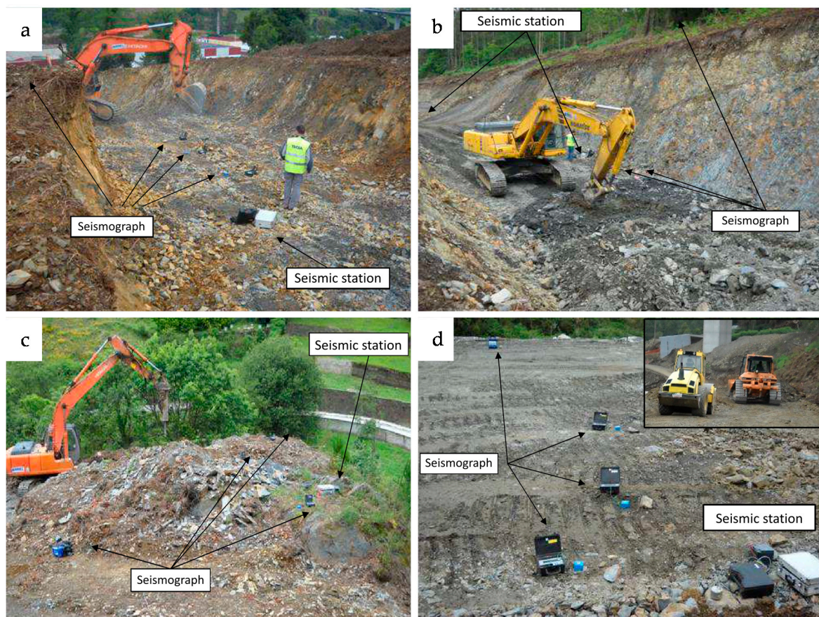
Figure 3. Layout of the equipment for monitoring the work of: (a) V-type bucket, (b) ripper (c) hydraulic hammer and (d) bulldozer and a vibrating roller.
