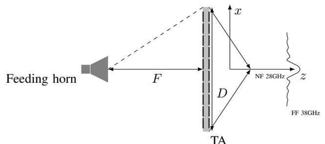
Fig. 1. Scheme of the Transmitarray antenna.
