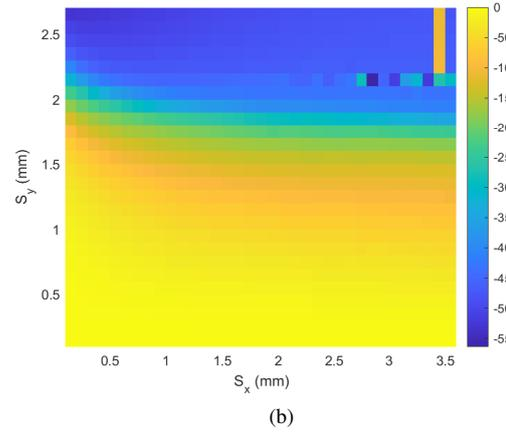
Fig. 4. Transmission coefficient simulated for the unit cell (38 GHz). (a) Module (dB). (b) Phase (degrees).
