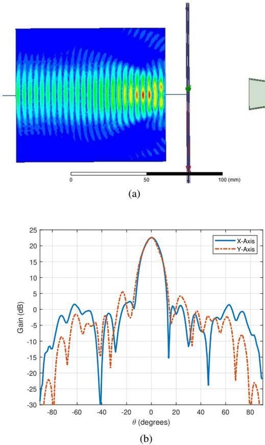
Fig. 8. TA simulation results (38GHz). (a) Near-Field. (b) Far-Field.
