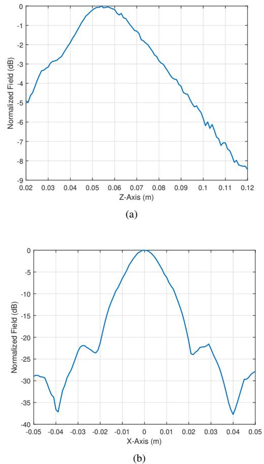
Fig. 7. Near-Field simulation results (28GHz). (a) Z-Axis. (b) X-Axis.
