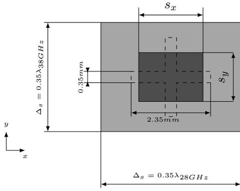
Fig. 2. Top view of the unit cell.
