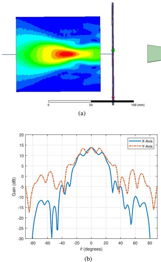
Fig. 6. TA simulation results (28GHz). (a) Near-Field. (b) Far-Field.
