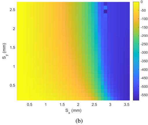
Fig. 3. Transmission coefficient simulated for the unit cell (28 GHz). (a) Module (dB). (b) Phase (degrees).
