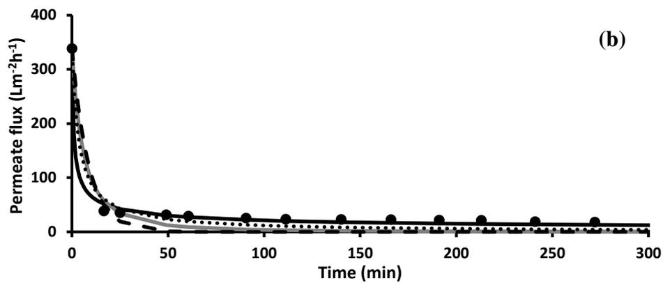
**Figure 4.** Evolution of the permeate flux (●) during the ultrafiltration of the mature (a) or young (b) leachate under VCR mode. Cake model (solid black line), standard model (solid grey line), complete model (dashed black line) and intermediate model (dotted line) predictions for each of them. In all cases: 1.6 bar, 70 °C, flow rate of 5.4 L/min and cross flow velocity of 3.2 m/s.
