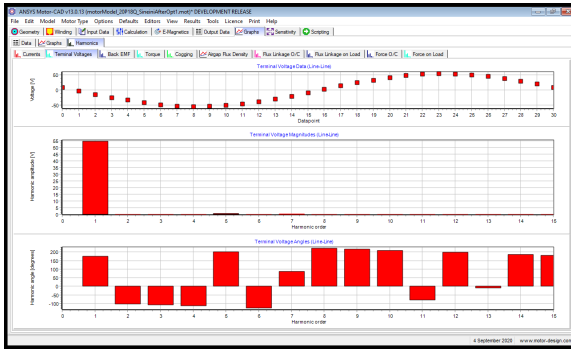
(g) Terminal Voltage Harmonics
