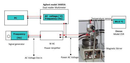
Figure 1. Schematic representation of the ohmic heating reactor.
