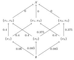
The optimal solutions of the shortest path problem are  $\emptyset \to \{x_2\} \to \{x_2, x_3\} \to \mathcal{X}$ and  $\emptyset \to \{x_3\} \to \{x_2, x_3\} \to \mathcal{X}$ , which correspond to the permutations  $\sigma_4 = (2, 3, 1)$  and  $\sigma_6 = (3, 2, 1)$ .
