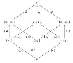
Solving the shortest path problem from  $\emptyset$  to  $\mathcal{X}$  using Dijkstra's algorithm, we obtain an optimal value of 2 that is attained with the following paths:
