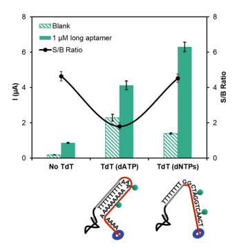
**Figure 3.** Chronoamperometric currents obtained without and with TdT amplification using only dATP or a mixture of dNTPs at 500  $\mu$ M concentration in the absence (striped bars) and in the presence (solid bars) of the long aptamer at 1  $\mu$ M and the corresponding signal-to-blank ratio at each condition.
