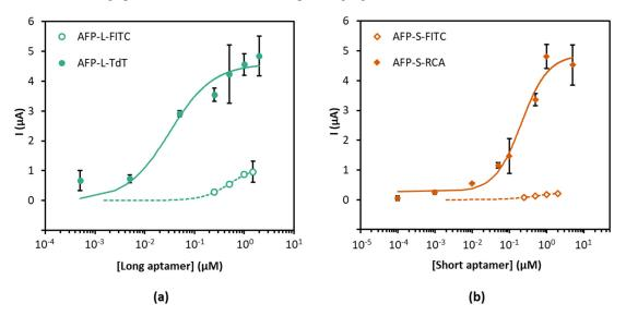
**Figure 4.** (a) Binding curves obtained on AFP-modified magnetic beads with the long aptamer without (open circles) and with (solid circles) TdT amplification. (b) Binding curves obtained on AFP-modified magnetic beads with the short aptamer without (open diamonds) and with RCA amplification (solid diamonds).
